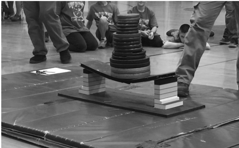
Figure 24 - Showing bridge, stanchions, plywood, gym pad and weights
